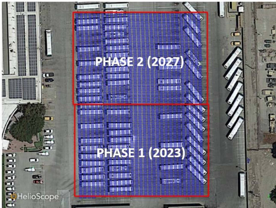
Figure 12-4: Pomona Depot Solar Layout
